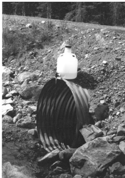
Figure 1. Mariotte bottle injecting into culvert.
